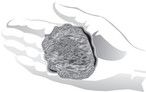
If the soil is powdery and will not retain the shape made by your hand, it is too dry. If it shatters when dropped, it is too dry.
