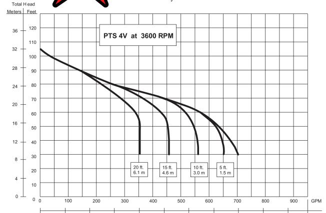
**Note** - The curve data represents the designed performance of the pump models, but does not take into account the many natural physical forces that act upon the pump in supporting the job. Contact Multiquip for detailed guidance and pump calculations for your specific application.
