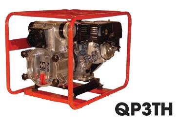
3" Suction/Discharge • 396 GPM Flow • 95' Head Moves up to 1.5" solids • Honda GX240, 7.9 HP
